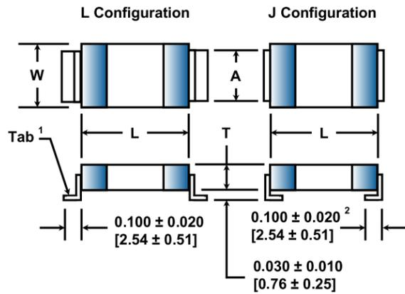
CalRamic Technologies LLC manufactures a series of highly reliable, military / commercial grade high voltage, surface mount, ceramic chip capacitors, that are intended for those applications where the assembly may be exposed to high levels of thermal and / or mechanical shock. Conservatively designed, they are ideal for use in demanding high voltage, high current environments.
