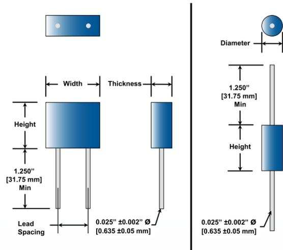
CalRamic Technologies LLC manufactures a series of highly reliable, encapsulated radial / axial leaded ceramic capacitors that are designed specifically for those severe conditions where the capacitor may be exposed to elevated levels of mechanical stress and high temperature conditions. These assemblies are packaged in a high resistance, high temperature rated case and backfilled with a high temperature epoxy that provides enhanced electrical isolation and added environmental protection.
