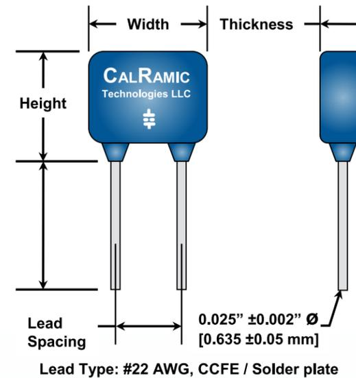
**CalRamic Technologies LLC** manufactures a series of highly reliable, mission critical, high voltage, radial leaded ceramic capacitors that are designed specifically for those non-repairable, space applications where the assembly may be exposed to high levels of thermal and / or mechanical shock.
