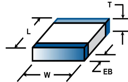
CalRamic Technologies LLC manufactures a series of highly reliable, mission critical, high voltage, multi-layer ceramic chip capacitors that are intended specifically for nonrepairable, space applications. Conservatively designed they are ideal for use in demanding high voltage, high current environments.
