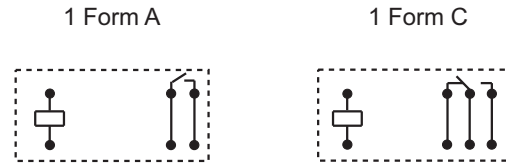
Wiring Diagram (Bottom view)
