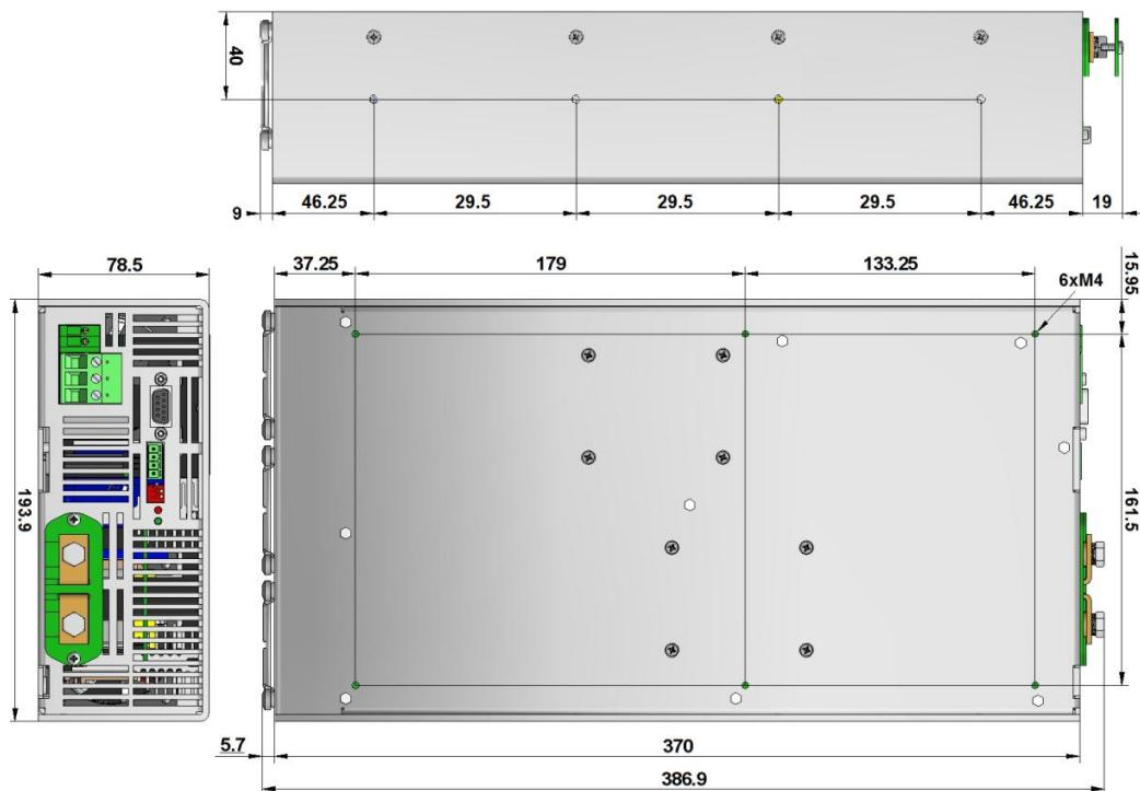
Maximum depth for the screws M4: 4.5mm
